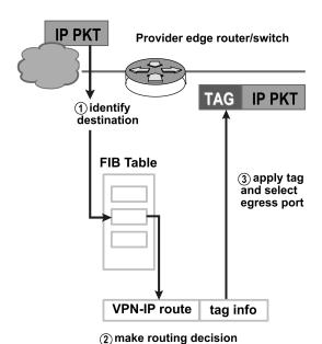
MPLS is an IETF standard technology that speeds up network traffic flow by avoiding packet analysis by intermediate routers (hops). This is done on the basis of so-called labels that are attached to packet by the edge routers of the backbone, on the basis of information stored in the forwarding information base (FIB). Labels are also used to implement virtual private networks (VPNs).
